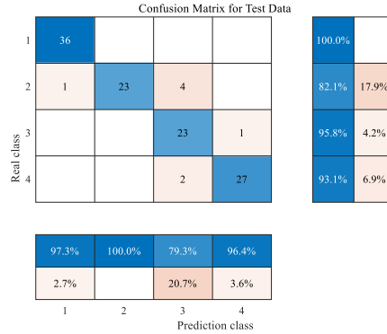
Figure 12: Single-cylinder stopping test set confusion matrix based on radial basis neural network
