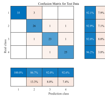
Figure 28: Confusion Matrix for Excessive Exhaust Valve Clearance Test Set Based on Radial Basis Neural Networks
