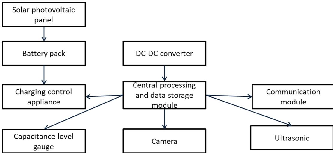
Figure 1: structure diagram of online water monitoring device
