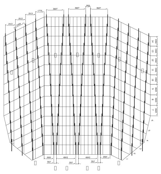
Figure 5: The distribution of support brackets for the grandstand countertops
