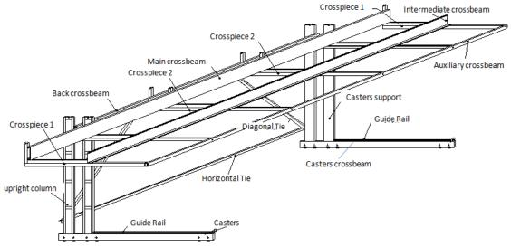
Figure 3: The stand Assembly without planking
