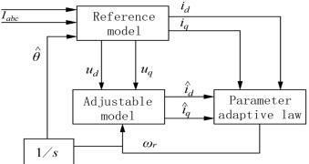
Figure 2: Schematic diagram of the system for MARS.
