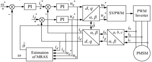
Figure 3: Design illustration of Sensorless vector control system of SPMAS based on MARS.
