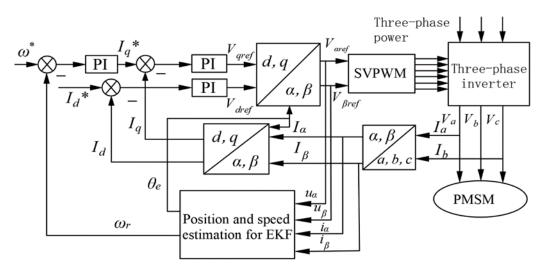
Figure 1: Design block of sensorless control system of three-phase SPMSM for EKF.
