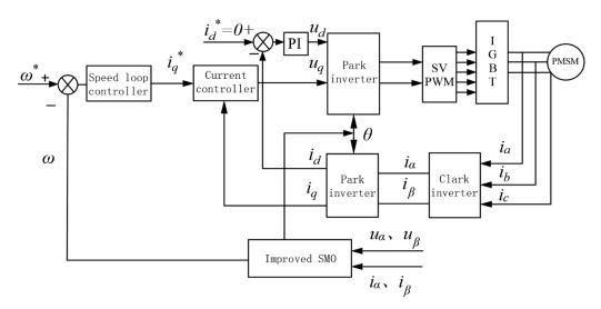
Figure 4: Design diagram of SPMAS control system based on improved SMO.
