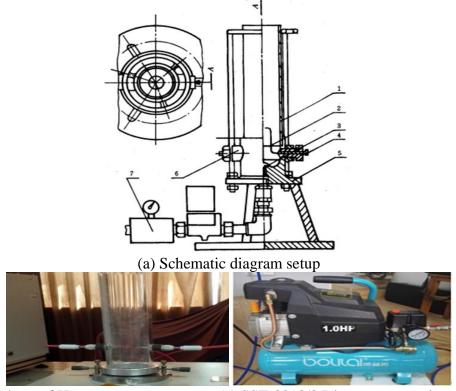
(b) The photo of Hartmann apparatus (c) SST-8010/8 Direct-connected compressor 1-quartz glass tube, 2-electrode, 3-diffuser, 4-steel bushing, 5-pedestal, 6-electrode socket, 7-storage tank
