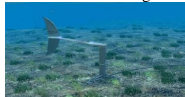
Figure9: Tidal energy turbine power generation system with bionic shark tail fin.
