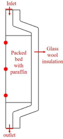
Figure 1: Schematics of the packed bed filled with paraffin spherical capsules. And top cut point (0, 0.42), center (0, 0.235) and low point (0, 0.05) are shown in the Figure.
