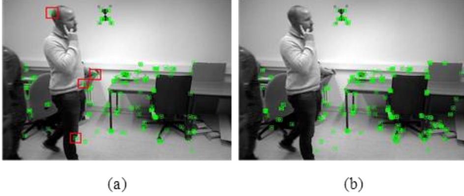
Figure 4: Demonstration of the Edge Feature Point Compensation Strategy.
