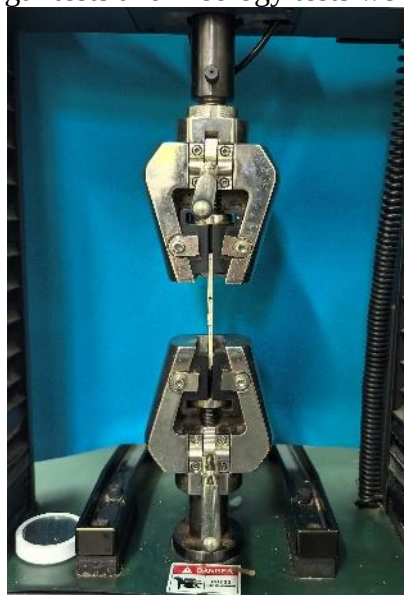
Figure 7 Testing process of dry adhesion strength on Universal Testing Machine.
