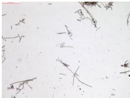
Figure 5: Fiber morphology of backing layers (100 $\times$ magnification)
