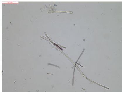
Figure 6: Fiber morphology of backing layers (200 $\times$ magnification)
