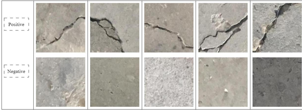
Figure 4 Concrete Crack Images for Classification Dataset
