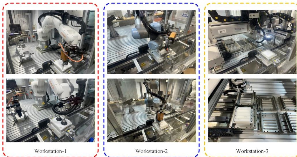
Figure 6: Battery module disassembly workstation
