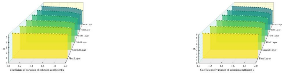
(c) The influence of the midpoint of the coefficient of variation of cohesion on the lower bound value of the reliability index
