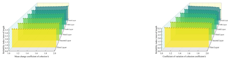
(a) The influence of the midpoint of the mean cohesion interval on the length of the reliability index interval (b) The influence of the midpoint of the coefficient of variation of cohesion on the length of the reliability index interval
