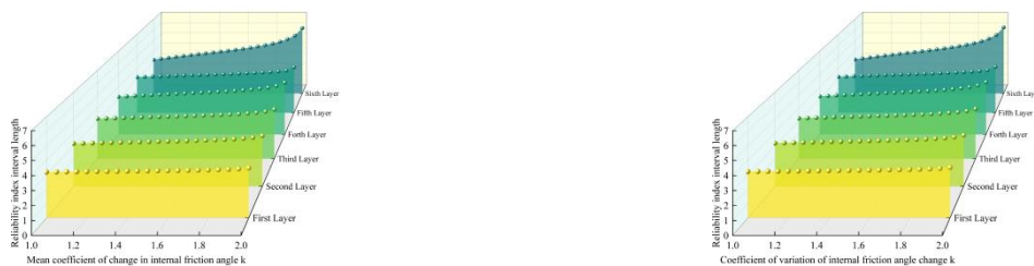
(a) The influence of the midpoint of the mean interval of internal friction angle on the length of the reliability index interval (b) The influence of the midpoint of the coefficient of variation of internal friction angle on the length of the reliability index interval
