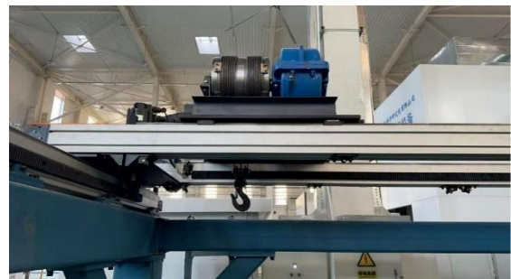
Figure 3 Hoisting-trolley fault-diagnosis test platform of the bridge erecting machine
