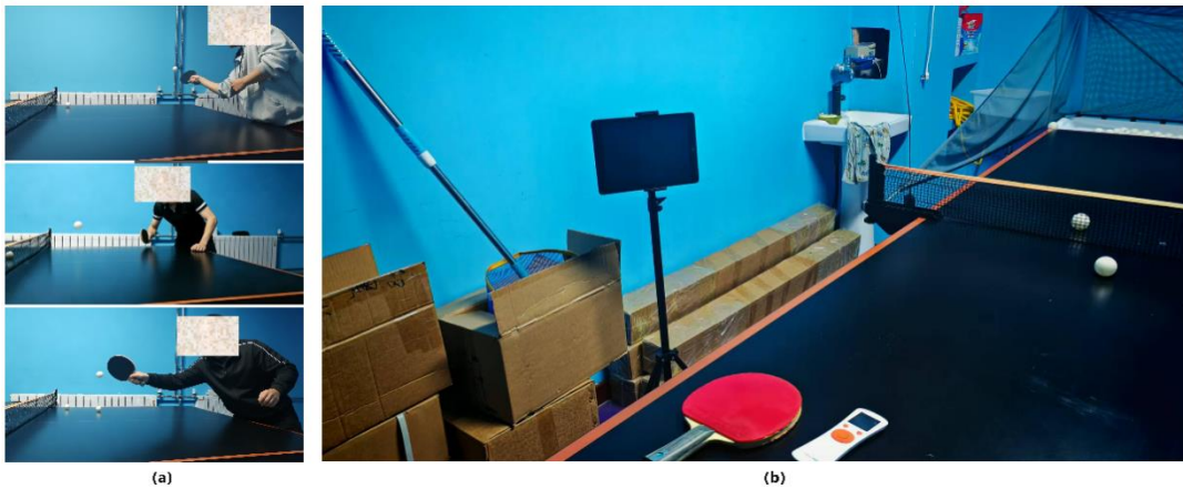
(a) Typical training scenarios of different participants; (b) Overview of the experimental platform, including the high-frame-rate acquisition device and display terminal.
